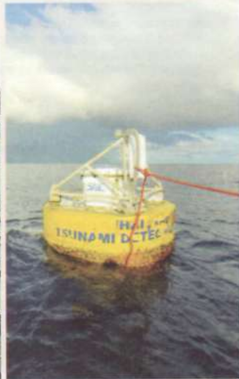
Fig. 1.14. Tsunami detection buoy
